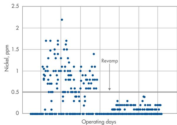
Figure 2: After the wash-oil zone revamp, the level of nickel in the HVGO fell.
