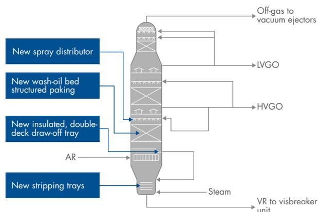
Figure 1: Modifications to the HVU included fitting a new spray distributor, new wash-oil bed structured packing and new stripping trays.
