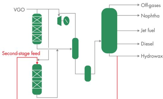
Figure 1: Before the revamp, the hydrocracker had a two-stage configuration. It was operating at 167% of the original design capacity and focused on middle distillate production.
