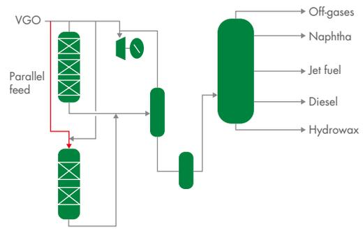
Figure 2: The revamped hydrocracker operates with the two original reactors in parallel. It has a feed rate of 300% of the design capacity and about 70% of its output is hydrowax, which is fed to the ethylene cracker.
