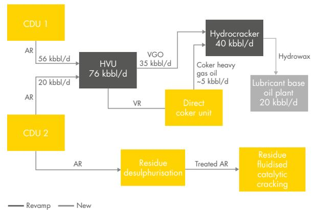
Figure 1: The refinery block scheme before (left) and after (right) the HVU revamp.
