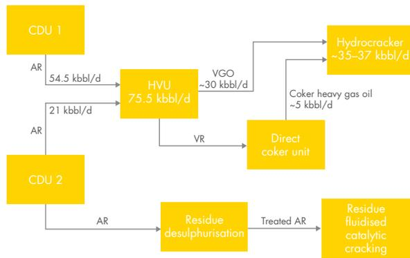
Refinery block scheme with new lubricant base oil unit
